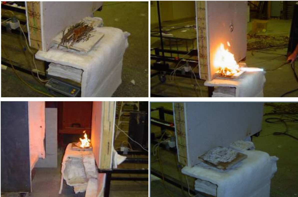
Figure 6.10 Determination of mass burning rate for debris when exposed to radiant heat: England et al (2008 11 )
